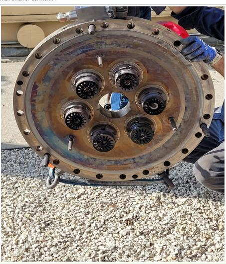
Off Site Primary, Secondary Nozzle, and Liner Refurbishment
