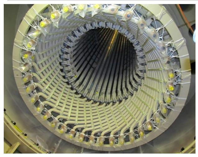
Stator windings are retained in the stator core by wedges.
